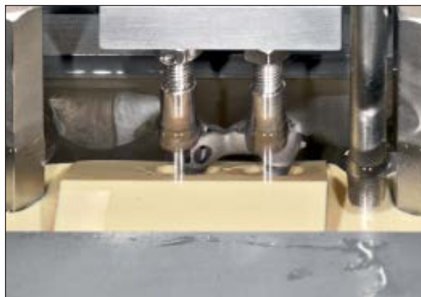
Fig 1 Sample of a Procera Implant Bridge directly fixed on the shoulders of two supporting implants and mounted in the water bath of a masticatory simulator at an angle of 135 degrees in relation to the long axis of the implants.
